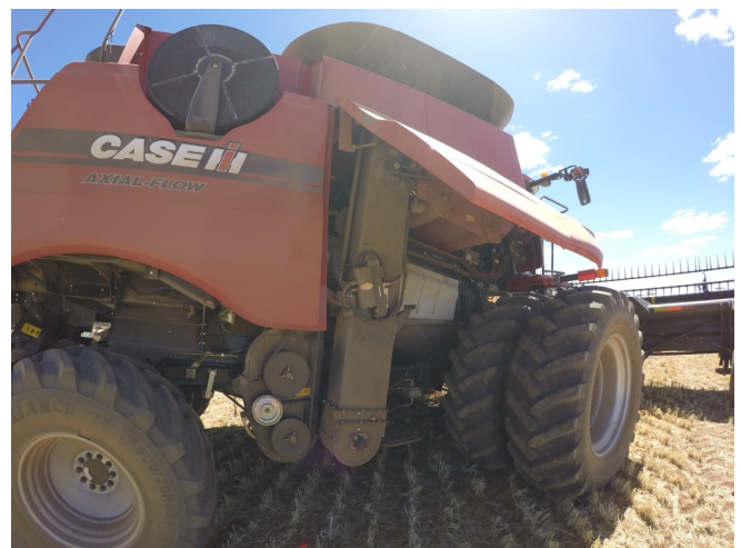
Figure 1. Picture of the CropScan 3000H Remote Sampling Head mounted to the clean grain elevator
