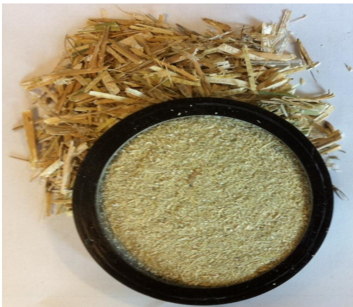
Figure2. Straw and ground straw in sample holder
